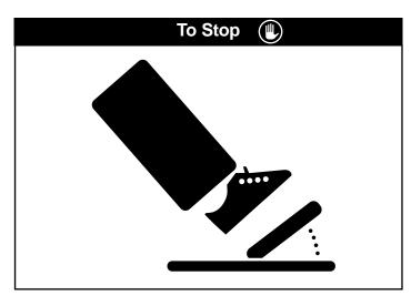
Your vehicle has a patented, electronic braking system that automatically stops the vehicle when your child's foot is lifted from the pedal.
